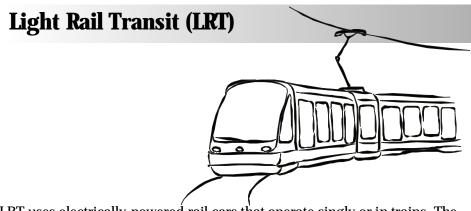
LRT uses electrically-powered rail cars that operate singly or in trains. The system moves more people faster than buses because LRT cars are larger than buses and run on dedicated tracks separated from traffic. LRT in the Broadway corridor would extend from Commercial Drive to UBC and would feature:
