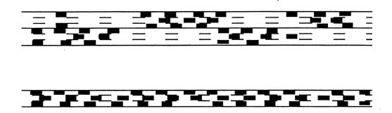
Because of this platooning effect, bridges with bridgehead traffic signals will have roughly half the vehicle capacity of similar bridges with free-flow approaches.
