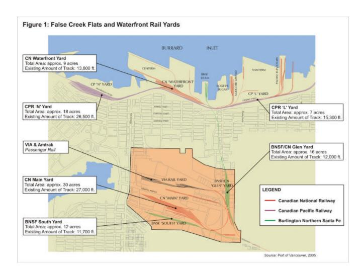
Along the Waterfront, CP uses its "N" yard for multiple purposes including Centerm container traffic and uses its "L" yard for grain trains and Vanterm container rail cars. CN uses its Waterfront yard for short term storage to serve nearby terminals, Centerm in particular.
