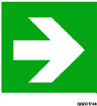
Figure A-3.4.5.1.(2)(c)-B “E005 Direction, arrow (90° increments), safe condition” symbol from ISO 7010
