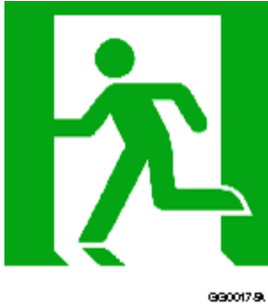
Figure A-3.4.5.1.(2)(c)-A “E001 Emergency exit (left hand)” symbol from ISO 7010
