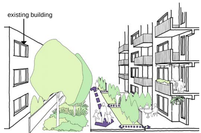
Figure 13. Illustrative example of a mid-block connection provided through an Enhanced Open Space Setback (EOSS) as part of a large, mid-block residential tower development.
