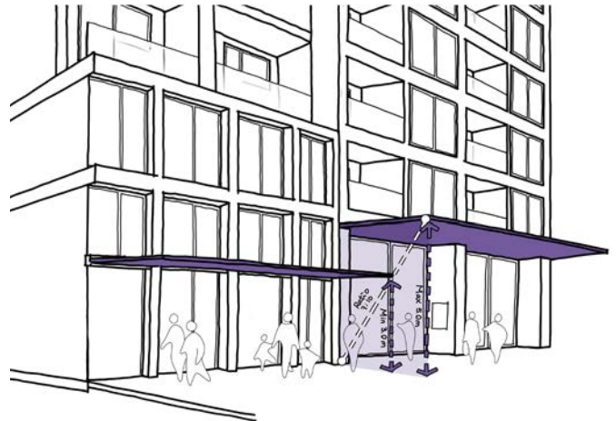
Figure 10. Diagram of desired weather protection height and proportions.
