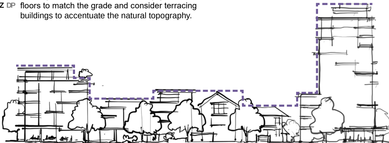
Figure 5. Creating sensitive transitions massing between building types.
