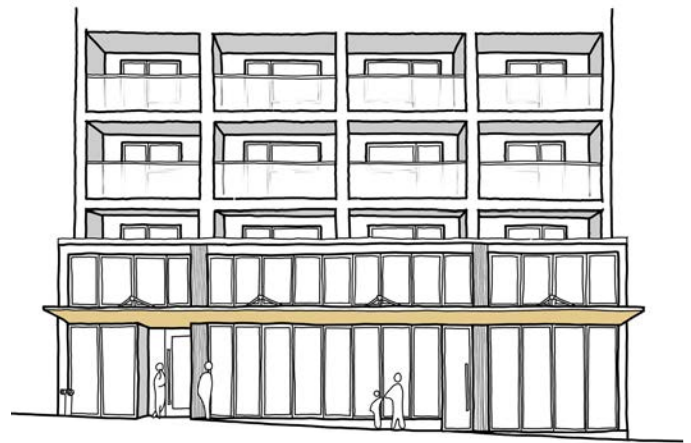
Figure 12. Door and window frames and wood soffits provide depth, thickness and a sense of warmth that enhances the pedestrian experience.
