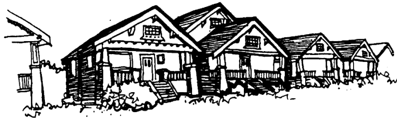
Figure 1 – Addition is set back from the front. This retains the original façade and minimizes disruption to the streetscape
