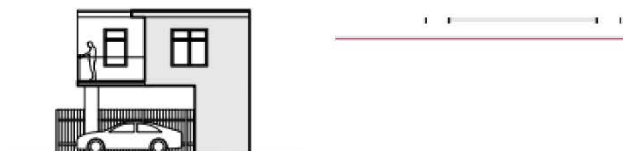
Figure 7 (Parking under second storey of infill building.)
