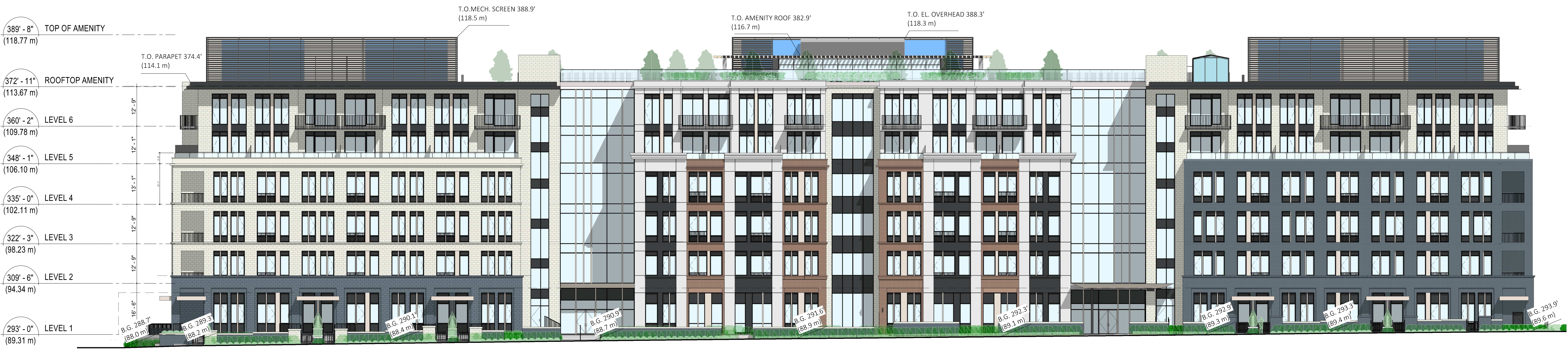
1 EAST ELEVATION (Facing Granville Street) 1/16" = 1'-0"
