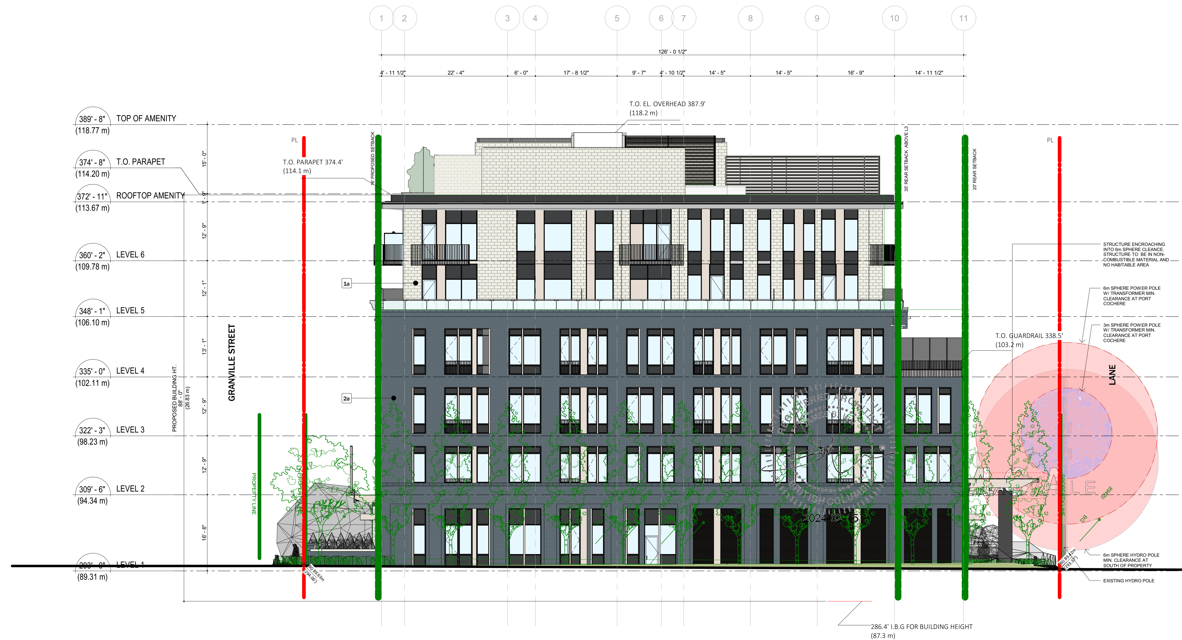
2 NORTH ELEVATION (Facing adjacent Property) 3/32" = 1'-0"
