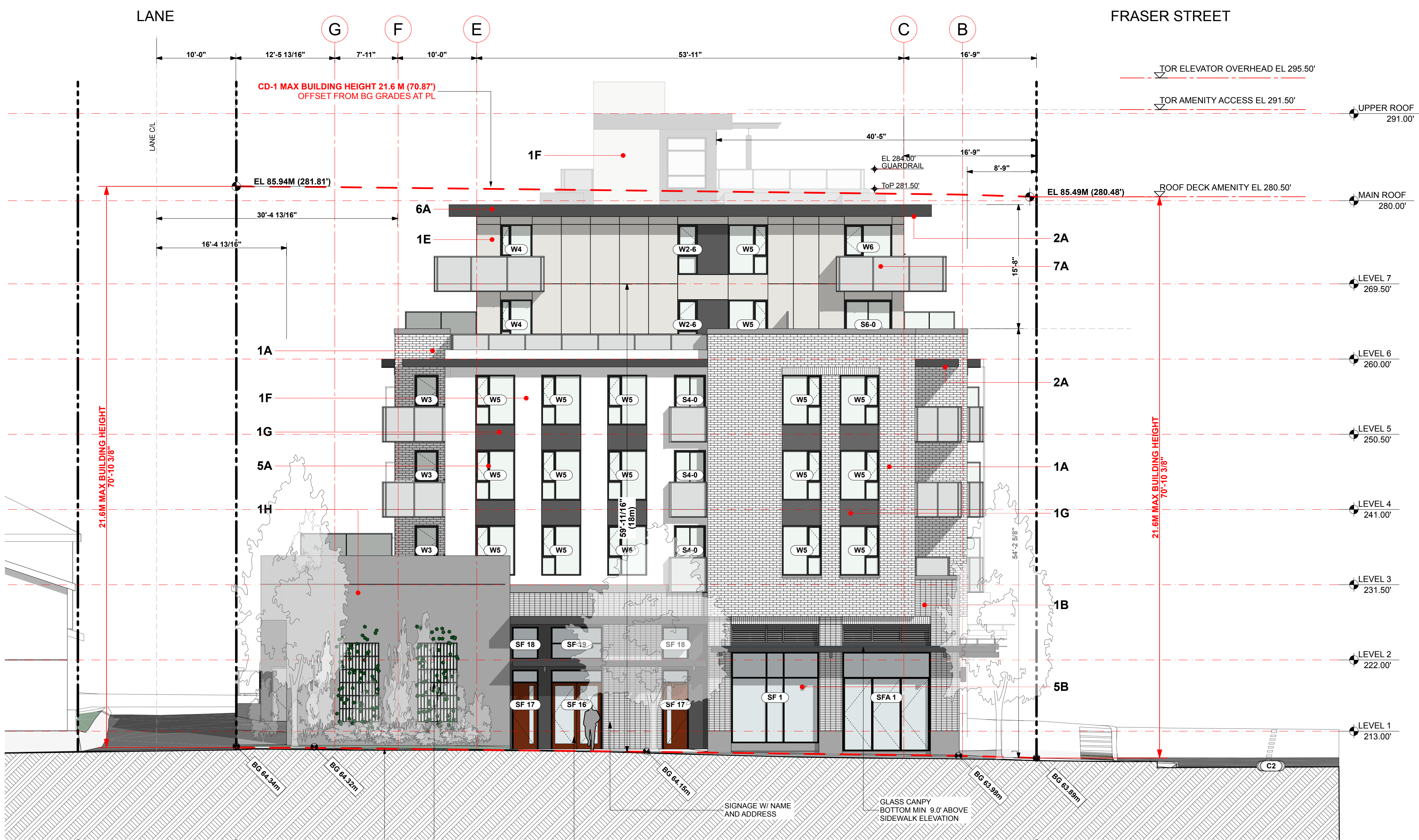
5 NORTH ELEVATION - E 28 TH AVENUE SCALE: 1/8" = 1'-0"
