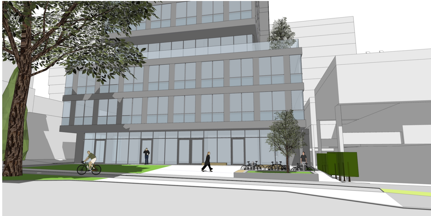
2. softscape area to the north of Tree #101 provides suitable area for water infiltration; new raised planter delineates edge of primary entrance plaza; short term bike parking located between the raised planter and building
