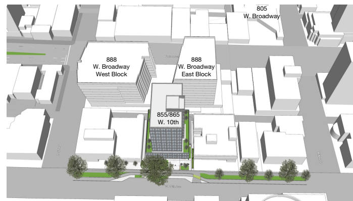
A. axonometric view of proposal from south showing the upper massing centred on the 3-storey podium; the majority of the midrise form of 855/865 W. 10th sits to the south of the raised courtyard of 888 W. Broadway, maximizing the views and privacy of both developments
