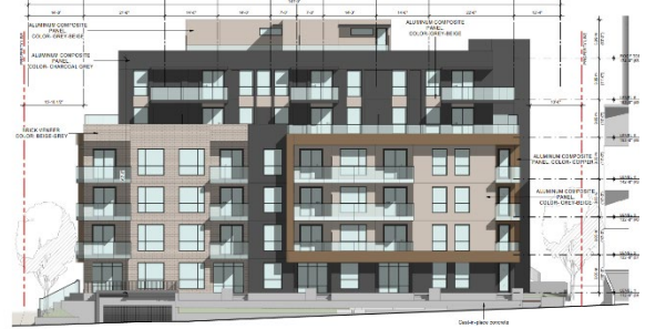
East Elevation (Rear)
