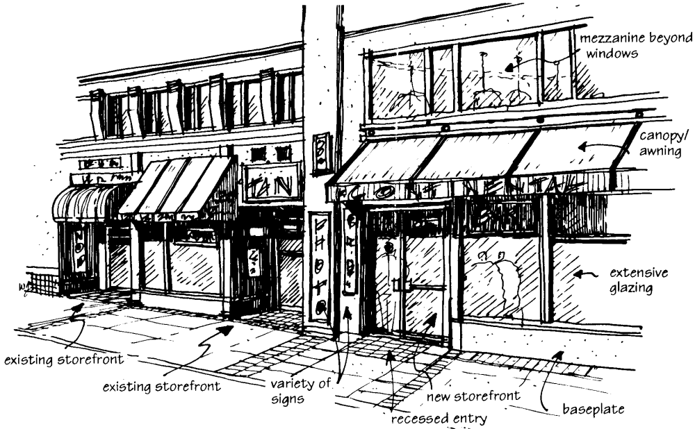
Figure 15. Traditional shop front configuration.
