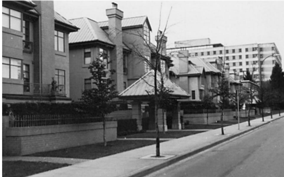
Figure 12. Long Facade Visually Broken into Components
