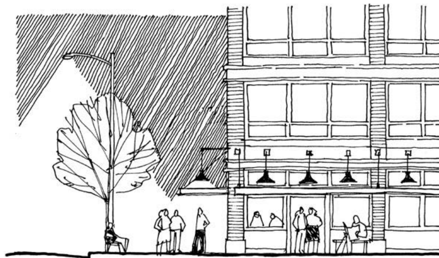
Figure 10. Illuminating building features can help create a sense of safe and intimate space around a building
