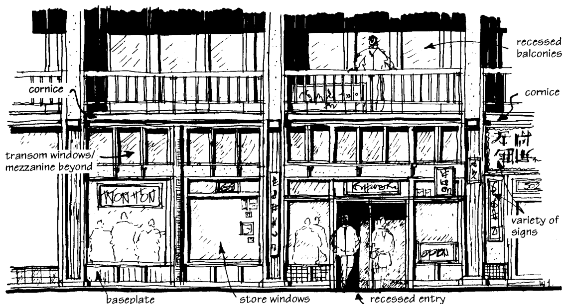
Figure 14. Typical lower Façade of heritage building.
