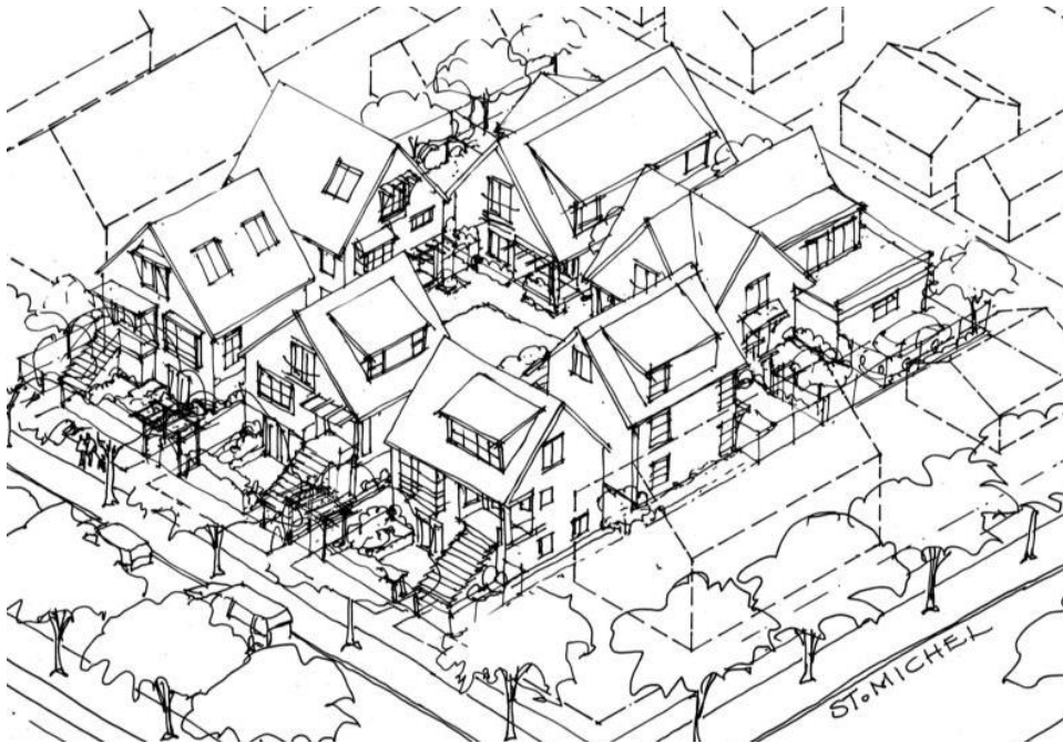
Figure 4: Cottage Development on Three 10 m (33 ft.) Lots or Two 15.24 m (50 ft.) Lots
