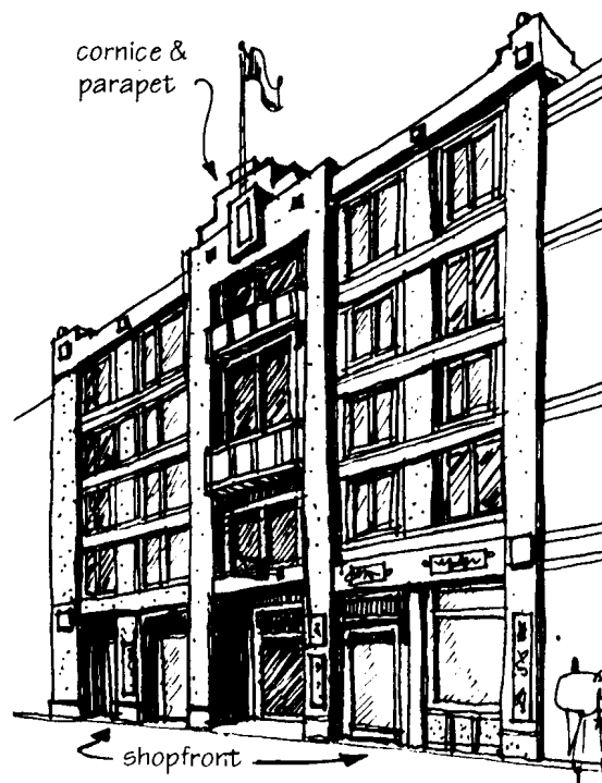
Figure 8. Vertical elements in facade composition
