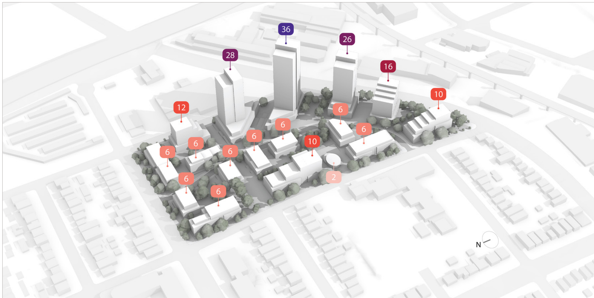
Optimum heights diagram (optimum heights are in storeys. See section 5.2.2 for policies relating to building variety and design.)
