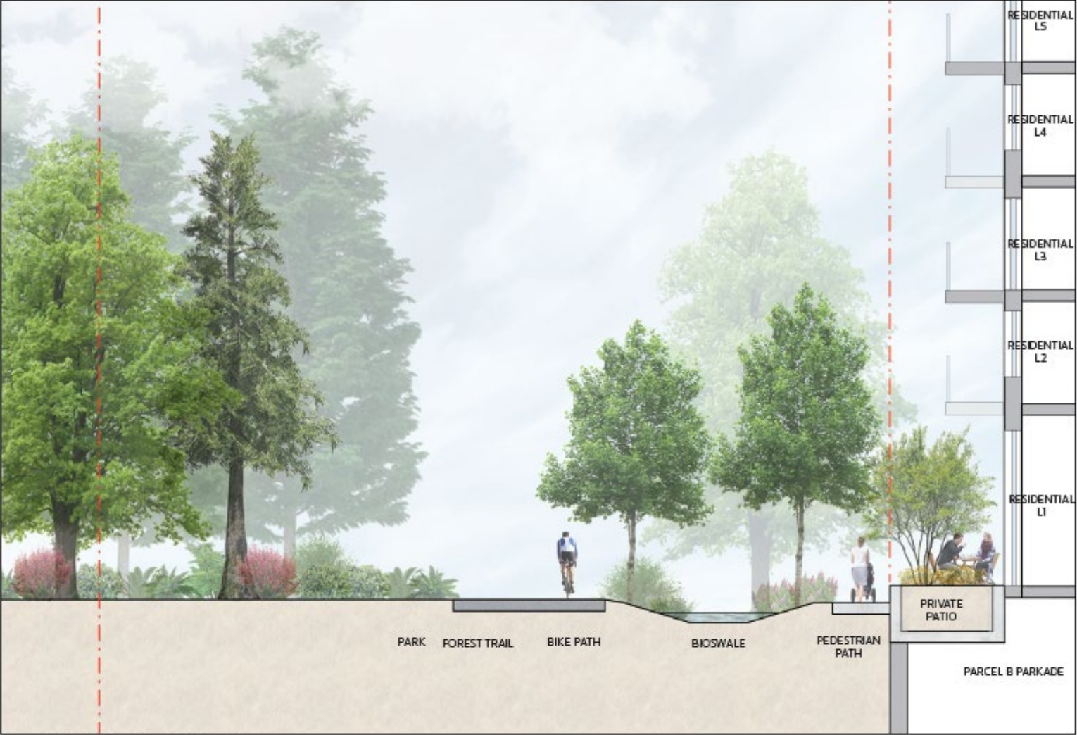
Figure 4-44: Heather Street ROW Section
