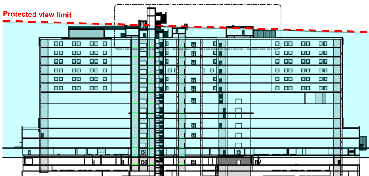
Figure 4: Section North-South Protected View
