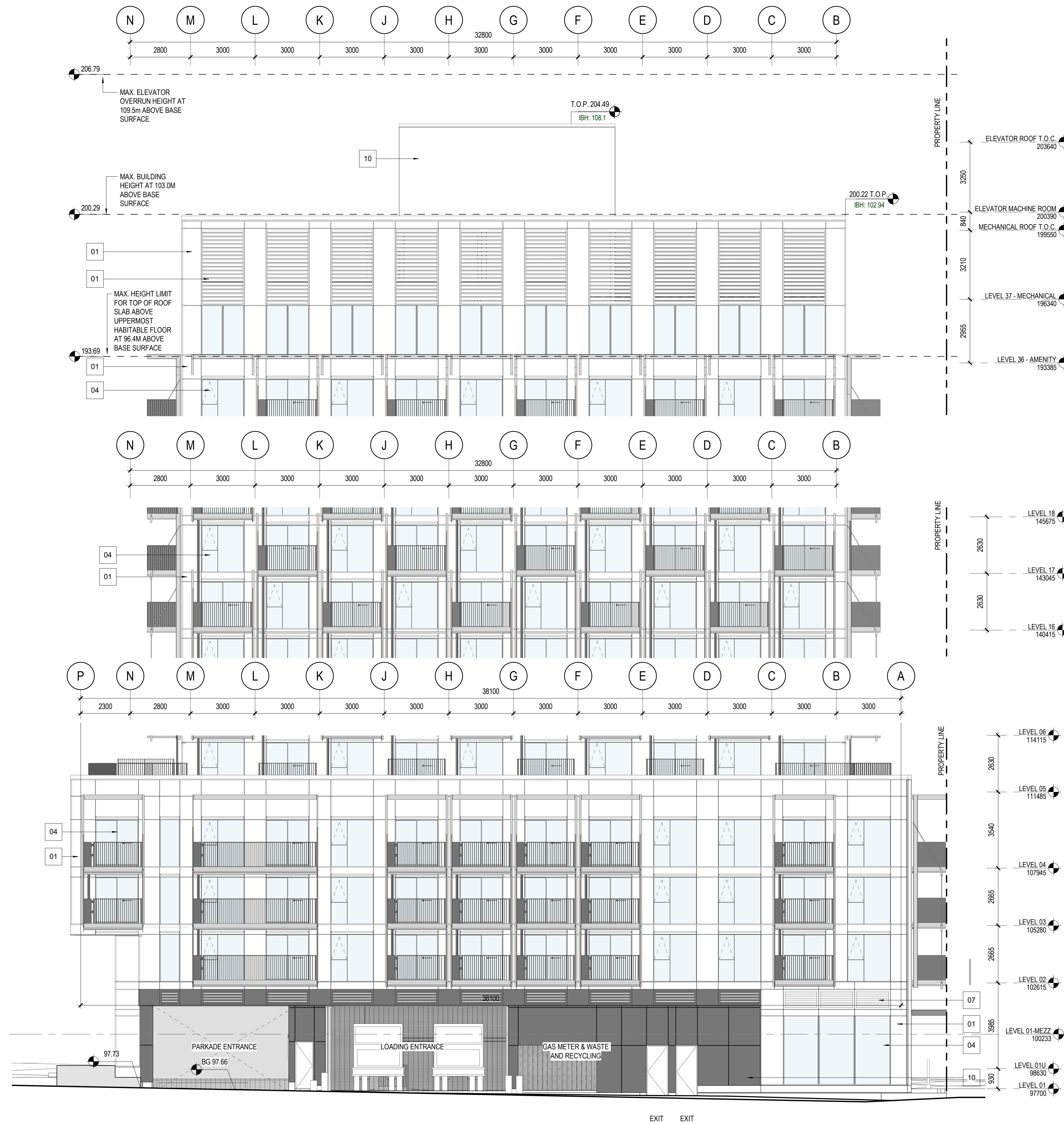
③ WEST ELEVATION - AMENITY & MECH ROOF 1:100
