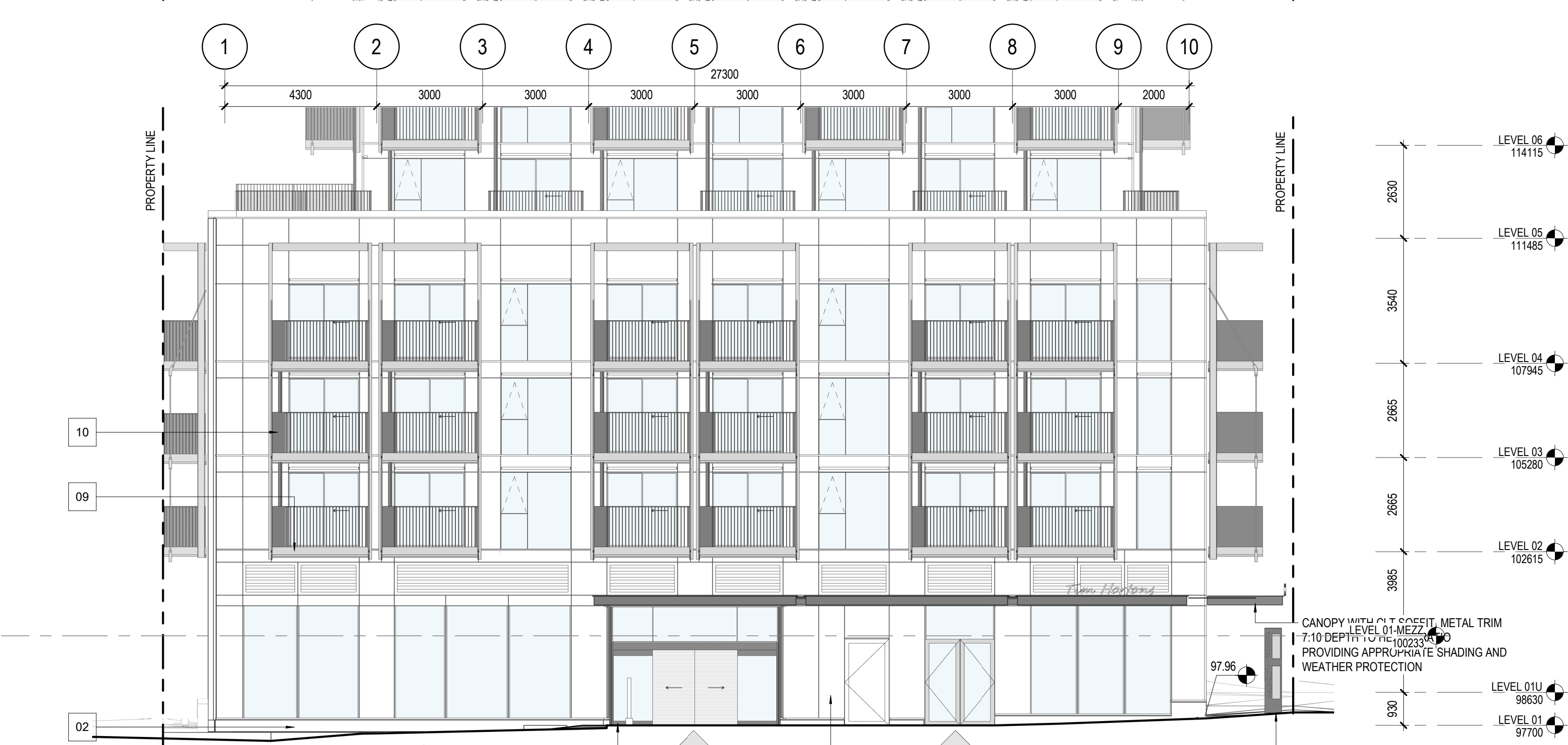
② SOUTH ELEVATION - TOWER 1:100
