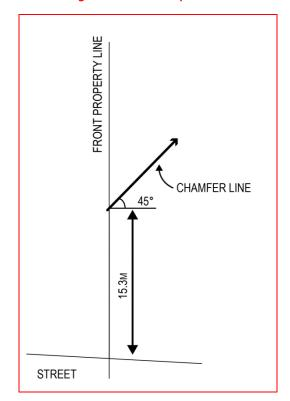
Figure 3. Chamfer Requirement
