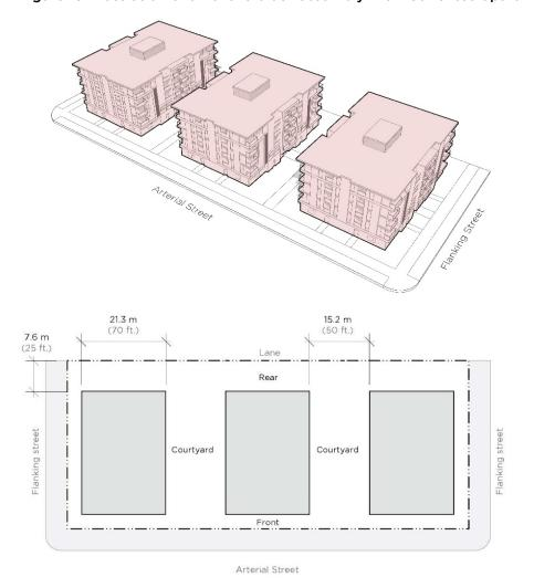
Reoriented apartment buildings may also be considered on partial assemblies if remaining lots are in a residential multiple dwelling district (RM or CD-1), and the internal side yard depth is increased to a minimum of 6.1 m (20 ft.); or if the assembly adjoins a T, L or H shaped lane where properties across the lane are oriented towards the flanking street.
