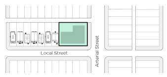
Figure 13: Illustration of a flanking corner site apartment with a wing extension
