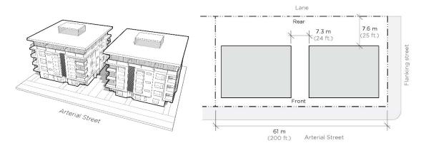
A single building may be considered on assemblies with a total site frontage less than 73.1 m (240 ft.) if a bridge element with a minimum width of 7.3 m (24 ft.) is included. This would provide sufficient vertical articulation to suggest the appearance of two distinct building forms to avoid a long, monotonous front elevation.
