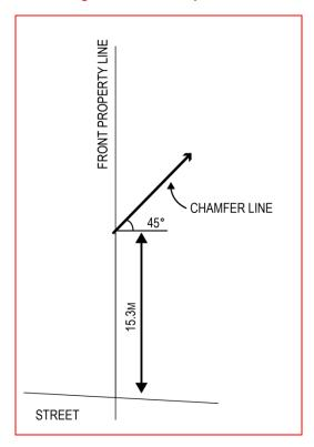
Figure 3. Chamfer Requirement
