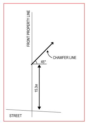
Figure 3. Chamfer Requirement
