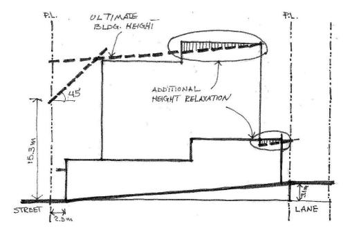
(d) For sites which slope across the frontage of the site, a minor height relaxation may be considered to allow a stepped building form, provided that the effect is not to significantly increase the overall pedestrian perceived building height above the maximum allowable building height.
