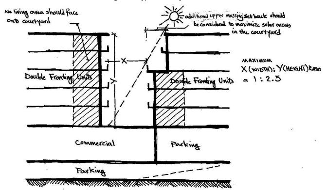
Figure 2: Typical Courtyard Section
