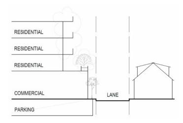
(a) For sites which slope upward from street to lane by more than 3.1 m, the 13.8 m portion of the height envelope may be measured from base surface.
