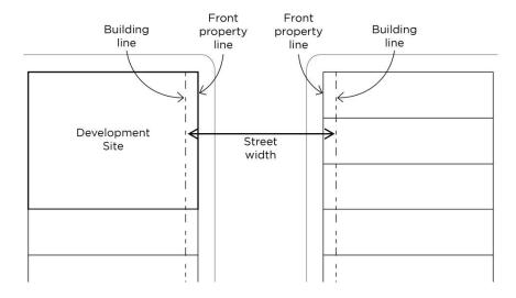
Where the 45 degree chamfer requirement does not apply, the building envelope shall be, as illustrated in Figure 18.
