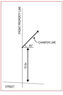
Figure 5. Chamfer Requirement
