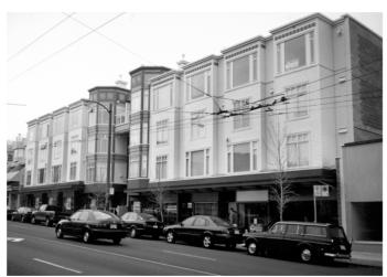
Figure 10: Example of broken massing on large frontage
