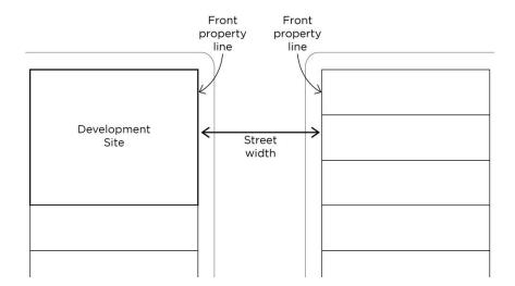
Figure 16: Street width measurement where no building lines exist
