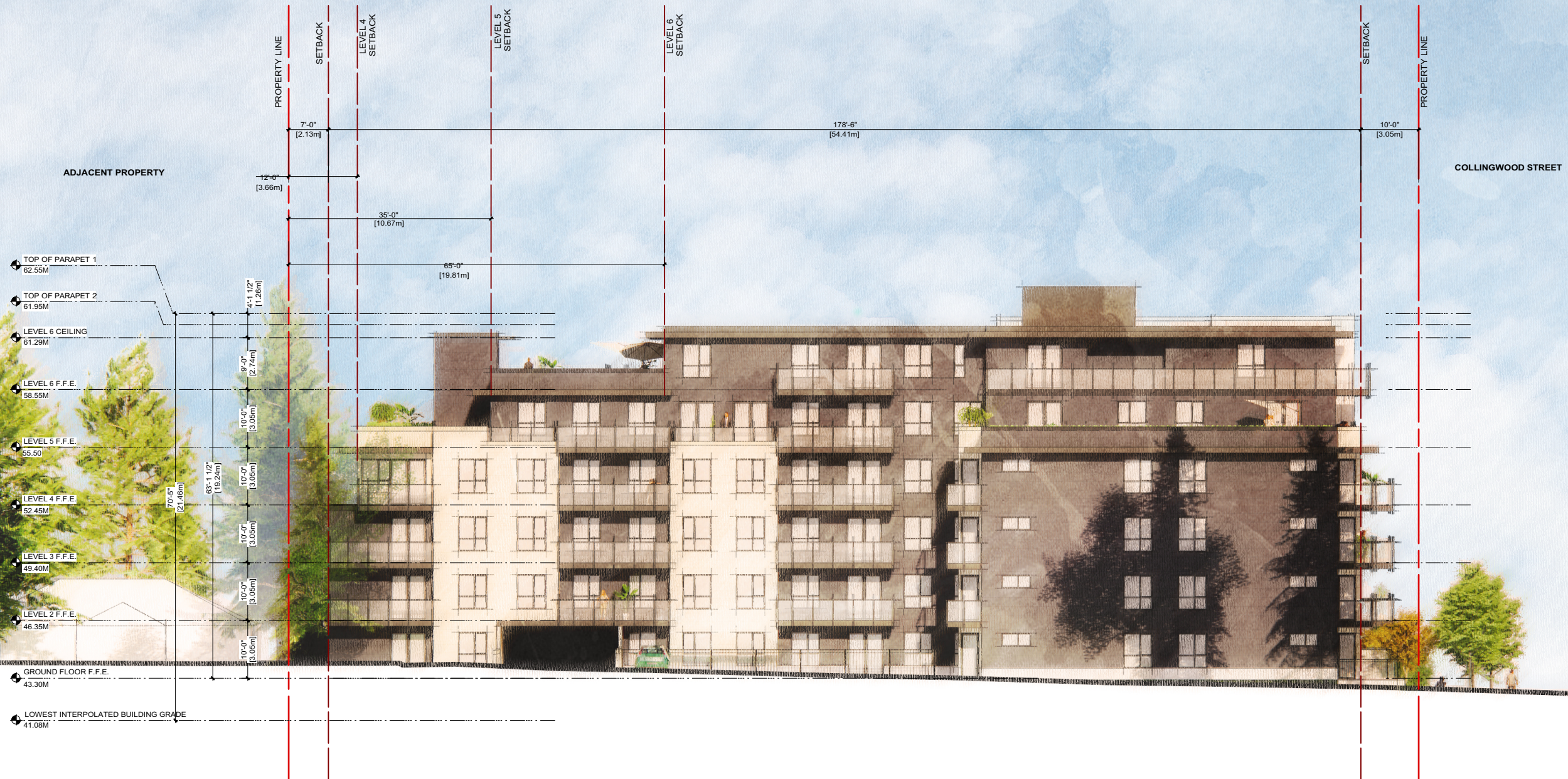
NORTH ELEVATION (COURTYARD) 1:250
