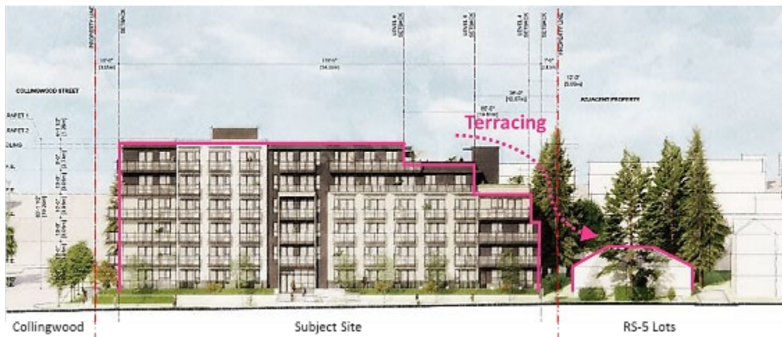
Figure 3: West 41st Avenue (South) Elevation
