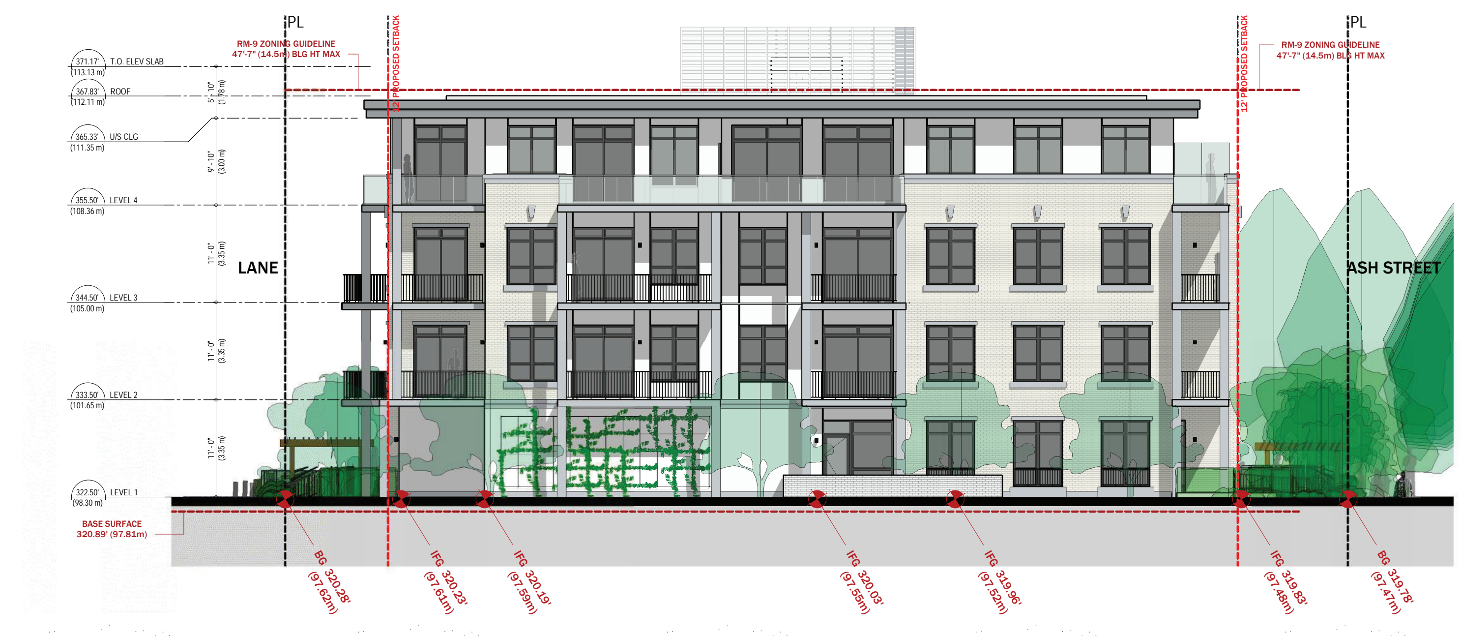
SOUTH ELEVATION - FACING ADJACENT PROPERTY - BUILDING 1
