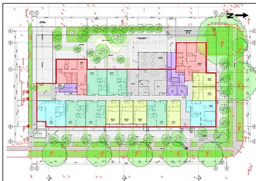
Figure 5: Proposed Ground Floor and Landscape Plan. Red-Line Indicates Typical Floorplate of Levels 2 - 4. Note the Retained Tree at the Northwest Corner
