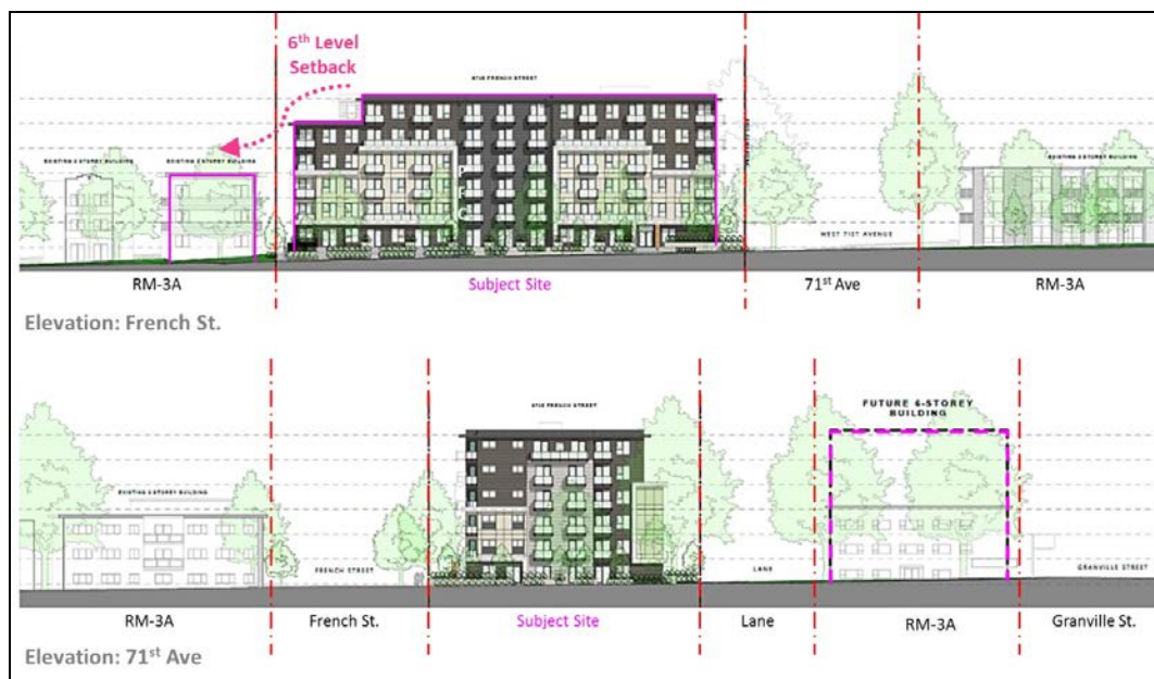
Figure 4: Top image: French Street Proposed Elevation Bottom Image: West 71 Avenue Proposed Elevation and Anticipated Six-Storey Forms Under the Plan
