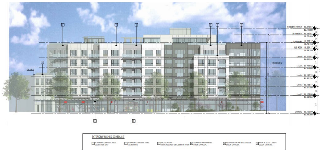
NORTH ELEVATION - KINGSWAY 3/8" = 1'-0" (ON 11x17)
