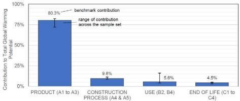
Figure 6: Embodied carbon breakdown by lifecycle stage. 68
