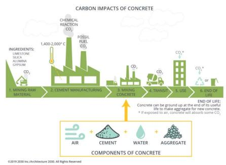
Figure 9: Emissions sources and sinks in the concrete lifecycle.<sup>73</sup>
