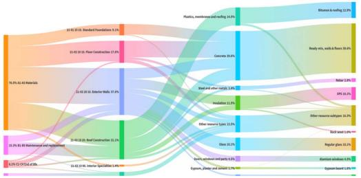
Figure 8: Breakdowns of embodied emissions from a low-rise wood-frame housing project by lifecycle stage, building element, material type, and product.<sup>72</sup>
