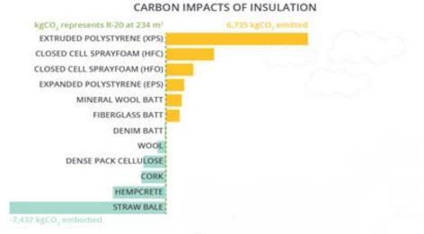
Figure 10: Relative emissions of insulation materials.74
