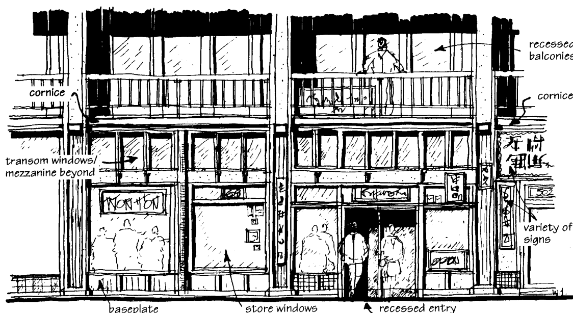
Figure 14. Typical lower Façade of heritage building.
