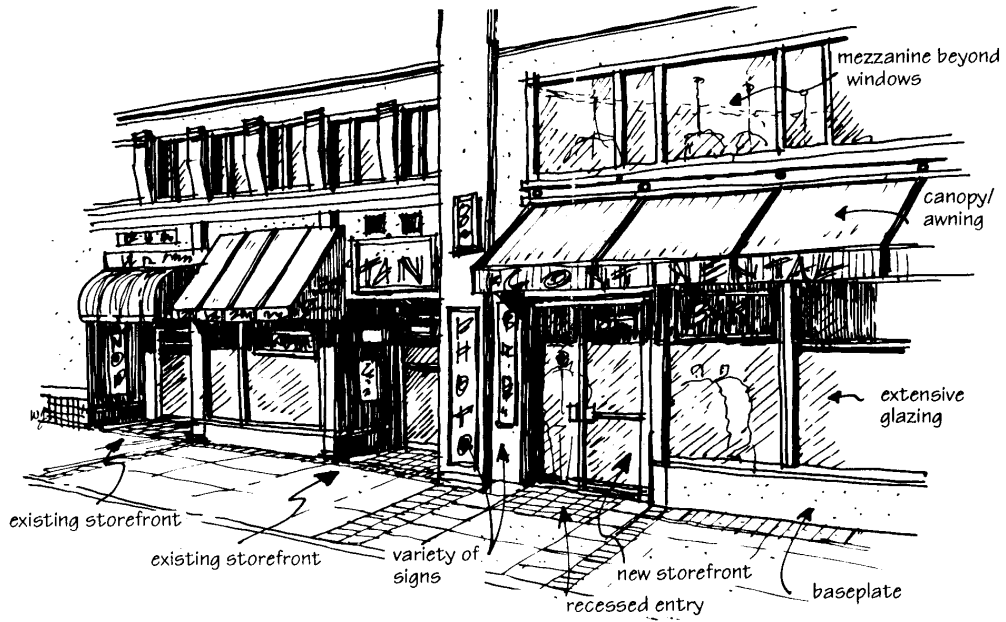
Figure 15. Traditional shop front configuration.
