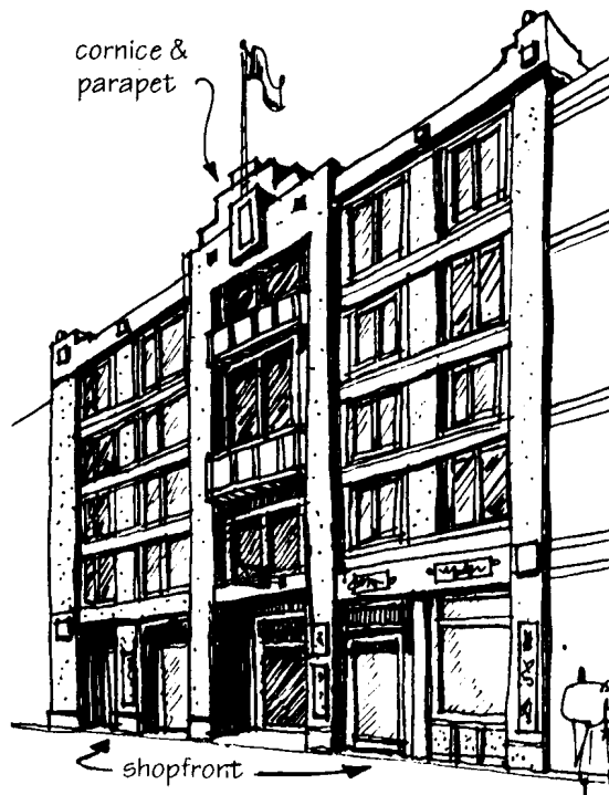
Figure 8. Vertical elements in facade composition
