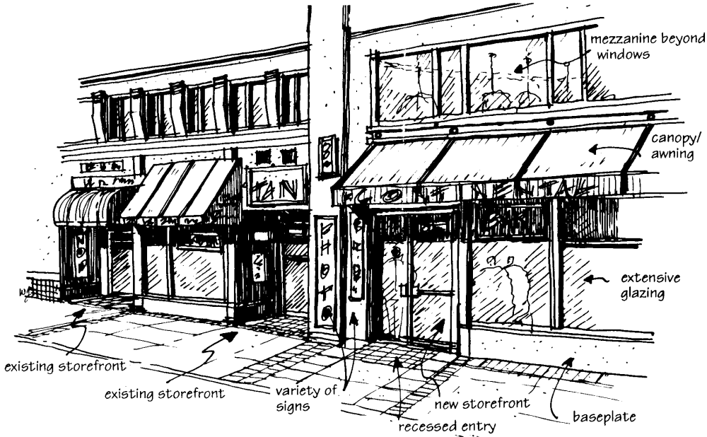
Figure 15. Traditional shop front configuration.
