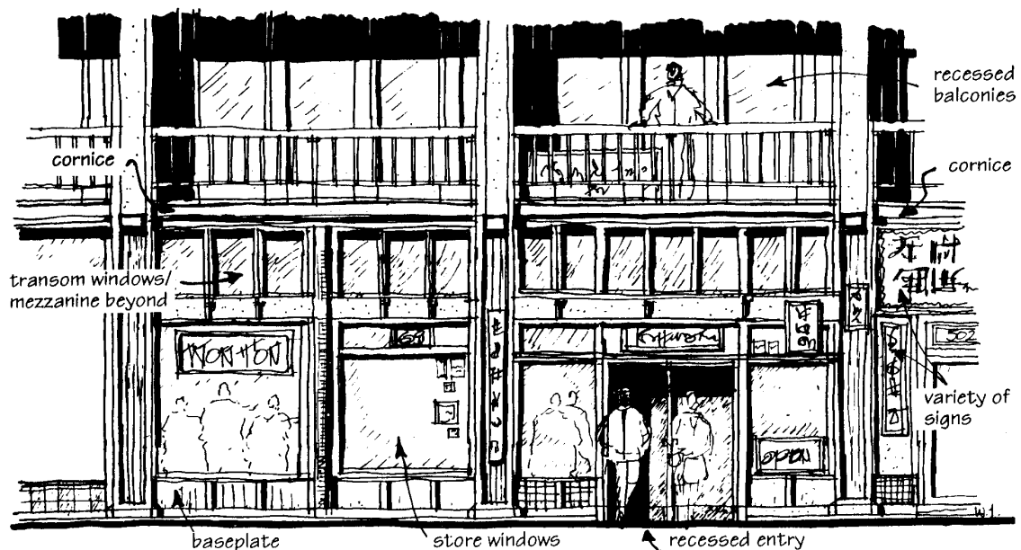
Figure 14. Typical lower Façade of heritage building.
