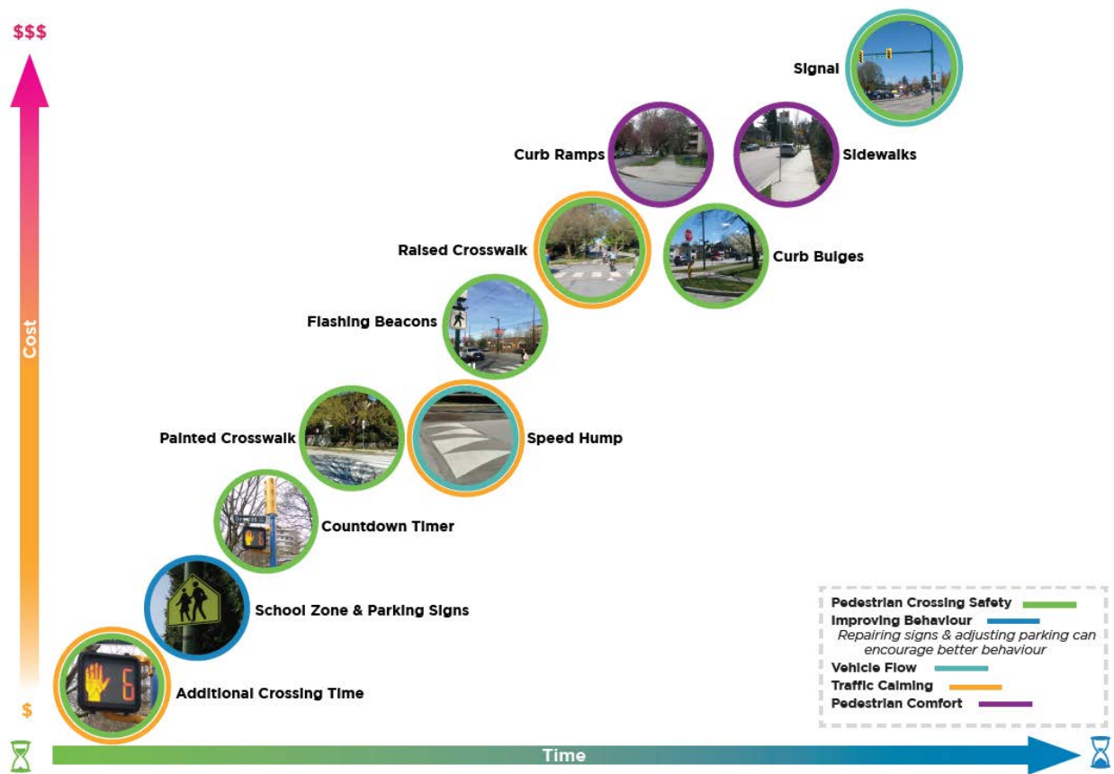
Figure 8. Infrastructure to Address Safety Issues Near Schools
