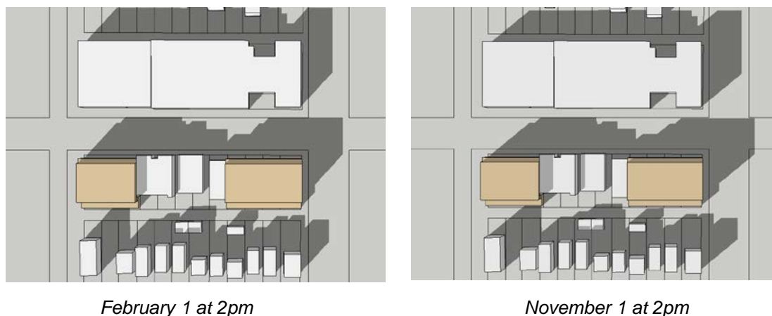
Figure 2. Shadow clears the sidewalk at 2 pm for development under C-2C
