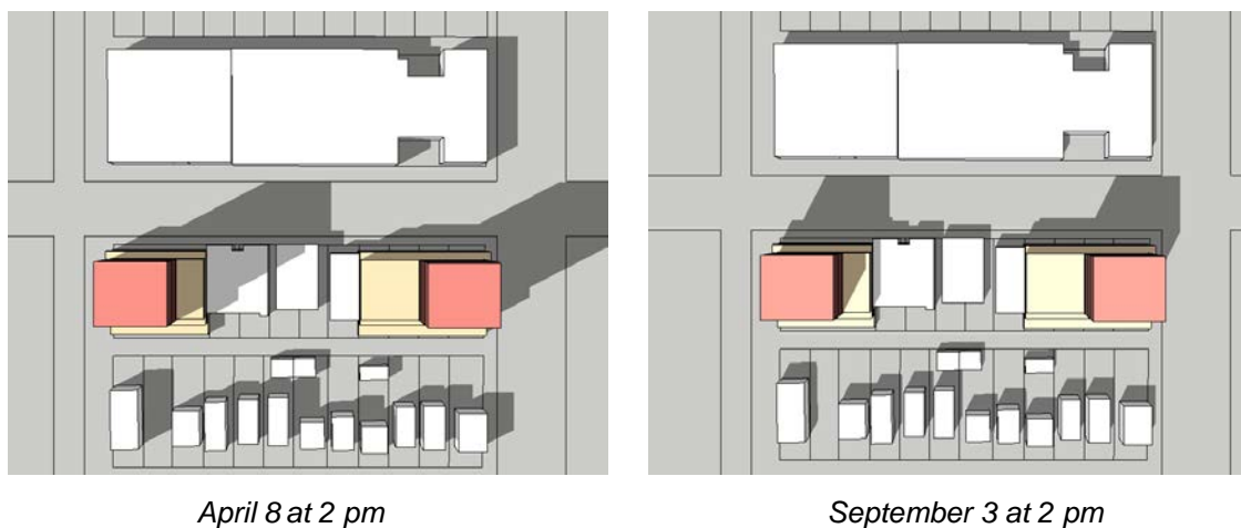
Figure 4. Shadow clear the sidewalk at 2 pm for proposed tower
