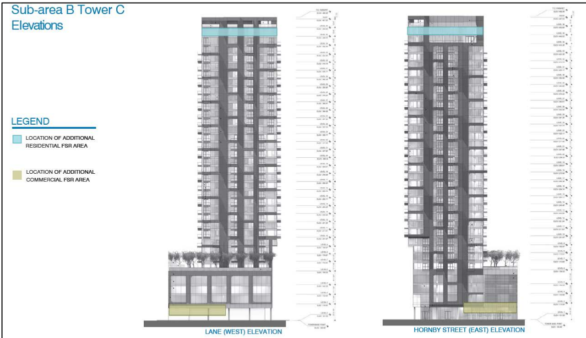
Figure 3: Elevation showing in blue proposed location of additional floor area in Sub-area B (Tower C)
