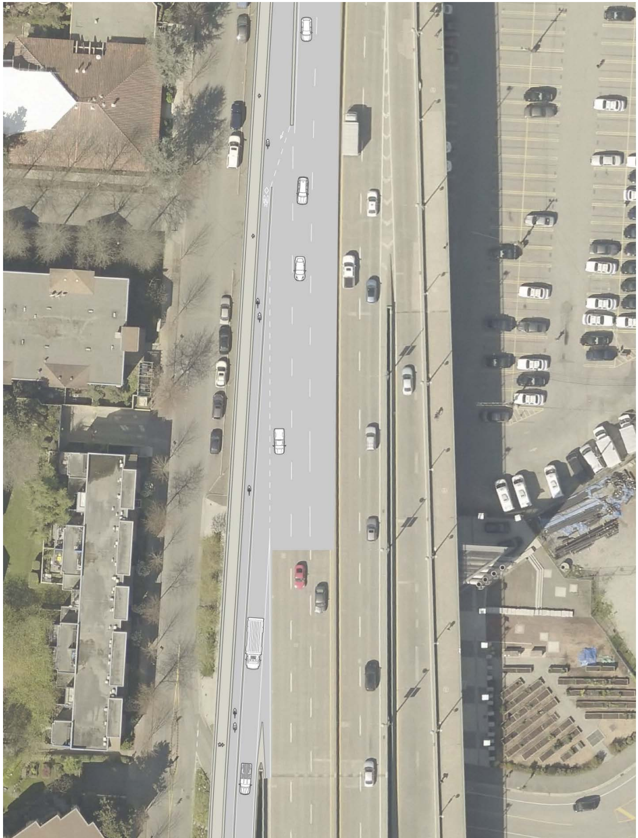
Figure 3: Transition at Top of Southbound-to-Westbound Ramp (Proposed)
