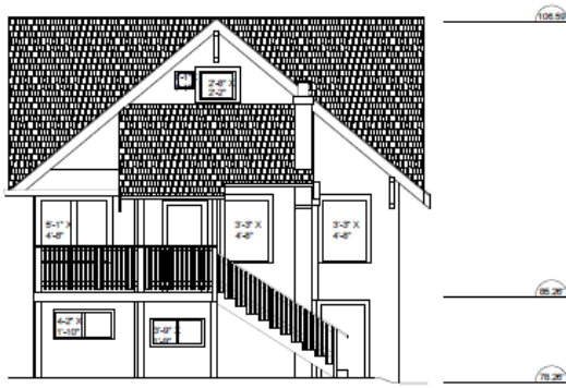
01 EXISTING EXTERIOR ELEVATION: SOUTH SCALE: 1/4" = 1'-0"
