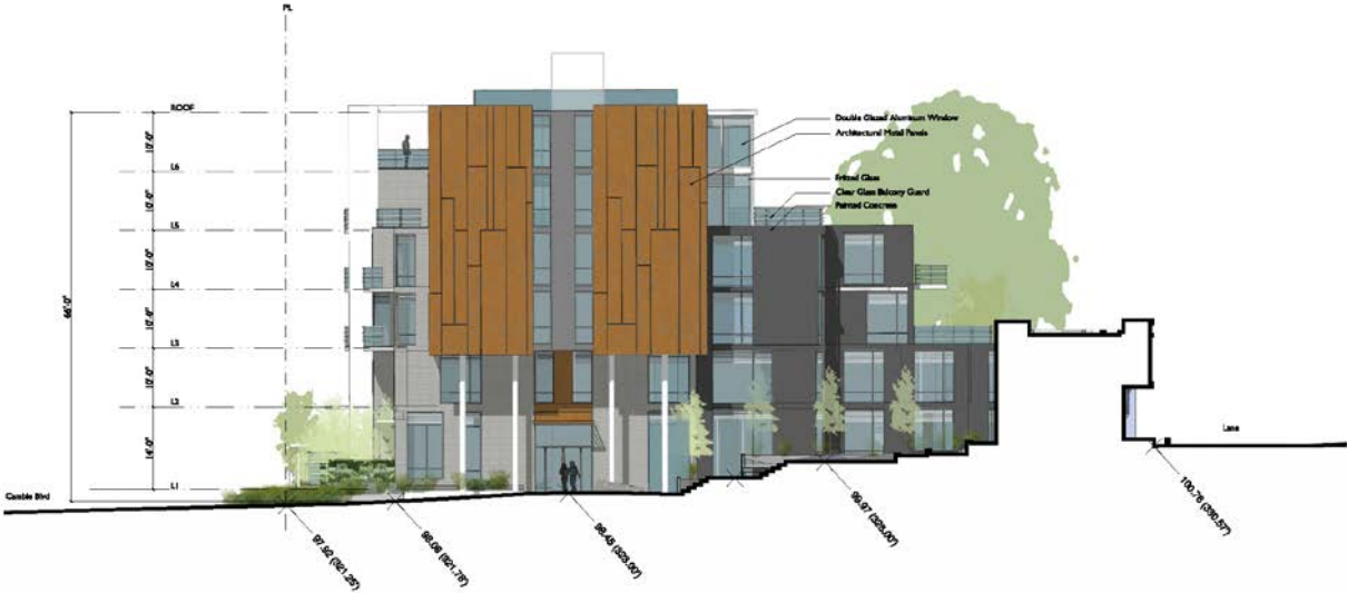
Building B South Elevation (from Building A/courtyard)
