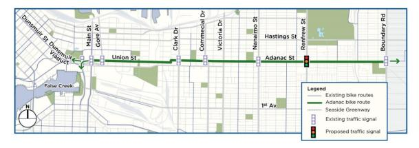
There are currently two crossings that are not signalized along the Adanac Bikeway: Victoria Drive and Renfrew Street. Staff are recommending that a signal be installed at Renfrew Street, as it is a 4-lane arterial crossing and removes an important barrier along the Adanac Bikeway. As the signal is installed, other street improvements are recommended, including modifications to the existing concrete median and new pedestrian curb ramps to meet accessibility guidelines.
