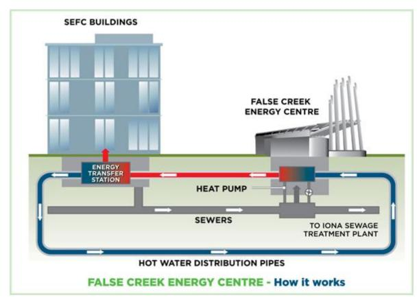
Figure 15.1 How the False Creek Energy Centre works
