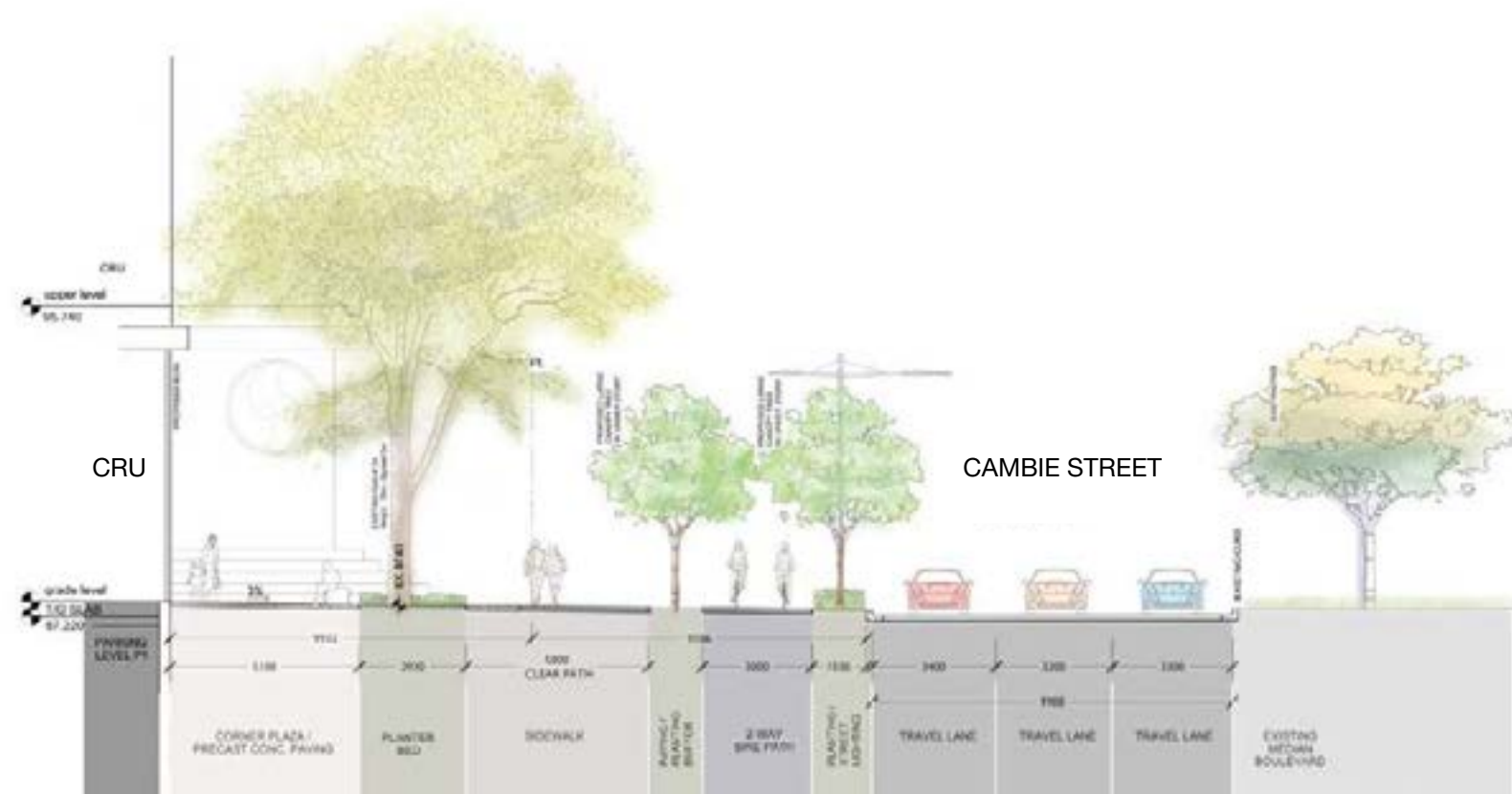
Section A Cambie Street near 45 th Avenue note: dimensions will be determined through detailed design
