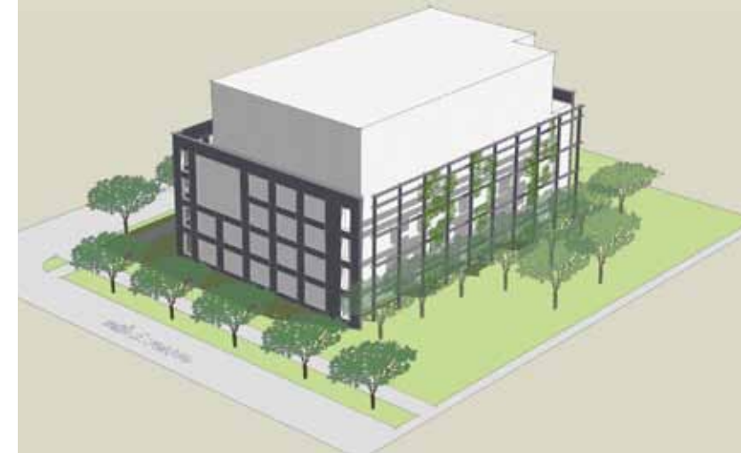
4. Layered Facade-Garden Screen at lane creates 4th floor stepback
