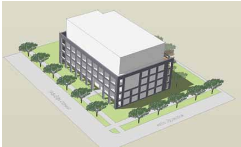
3. Layered Facade - Masonry Screen on Cambie to articulate the four storey streetwall and to create the step back
