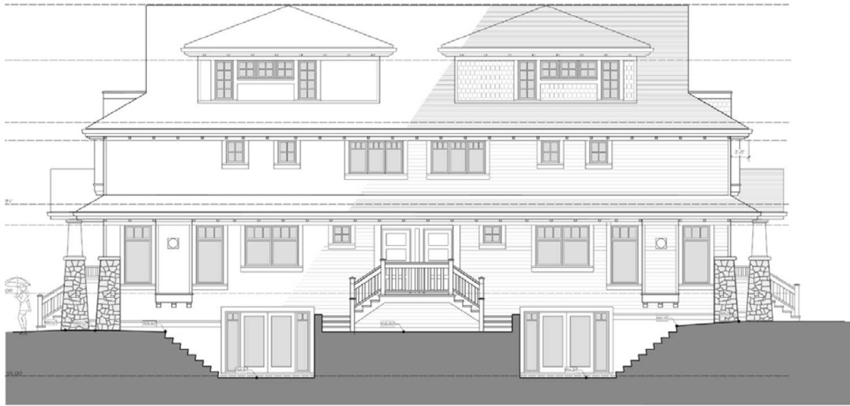
South Elevation – of principal building, showing secondary suites' exterior access at basement level
