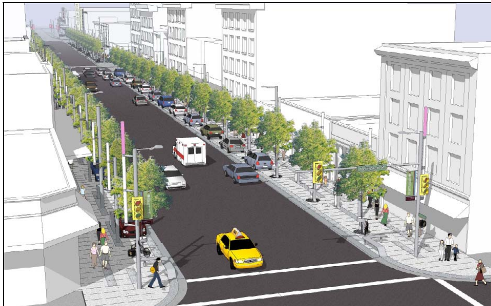
Figure 1 - Perspective Drawing Illustrating Sidewalk Parking Stalls
