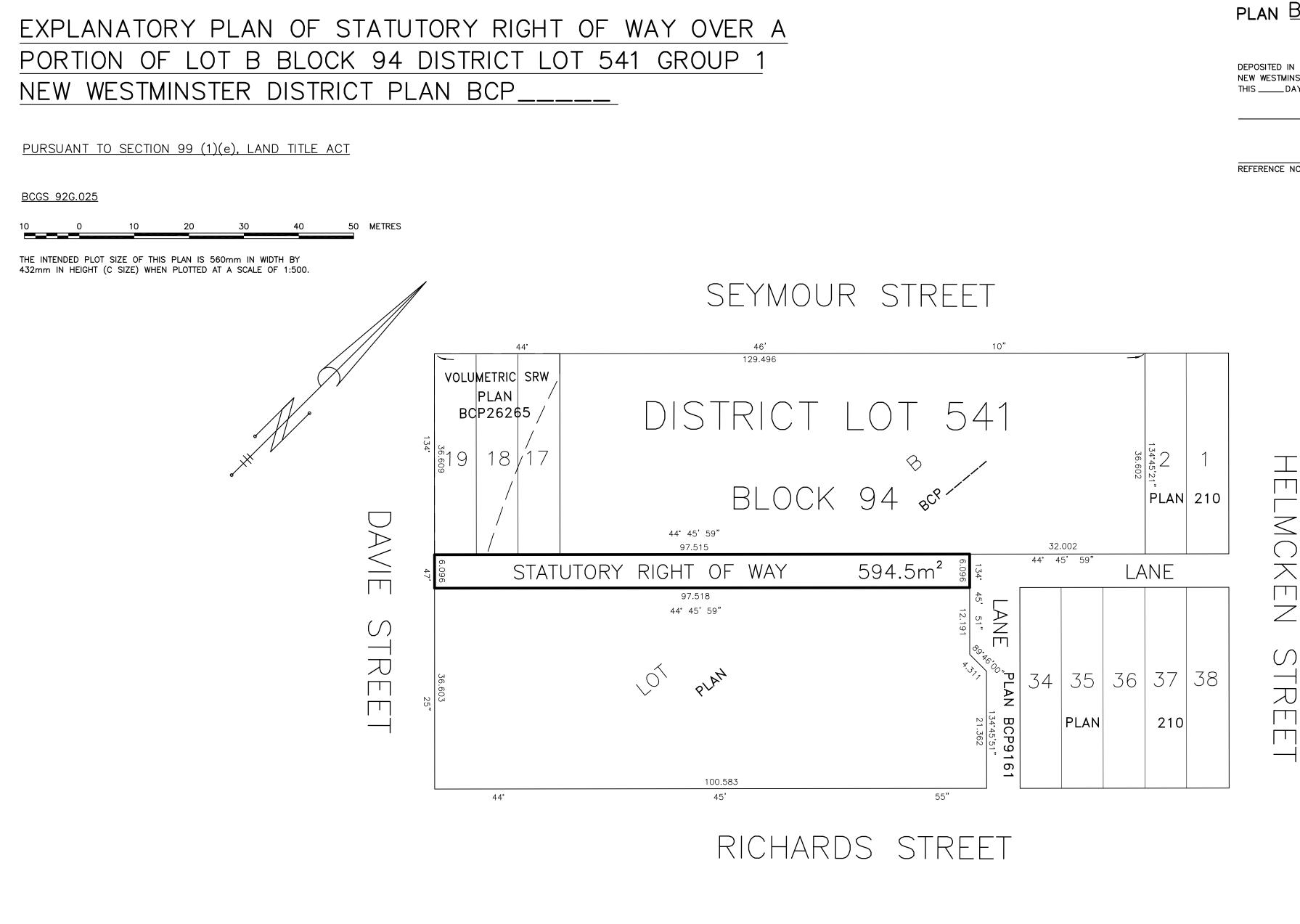
INTEGRATED SURVEY AREA 31, CITY OF VANCOUVER, NAD83 (CSRS). GRID BEARINGS ARE DERIVED FROM PLAN BCP\_\_\_\_
