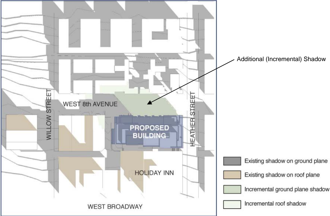
Figure D5 – Shadow at 10:00 a.m. during equinox (March 21st and September 21st)
