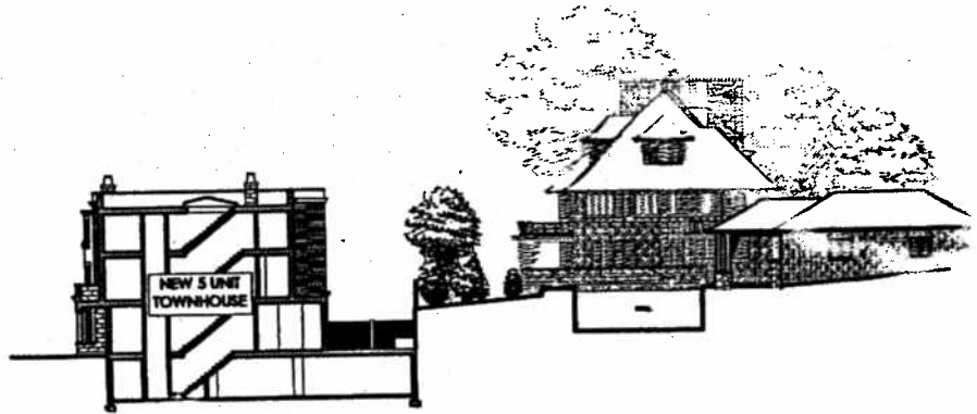
3 PROPOSED SECTION AT HERITAGE HOUSE REAR WING
