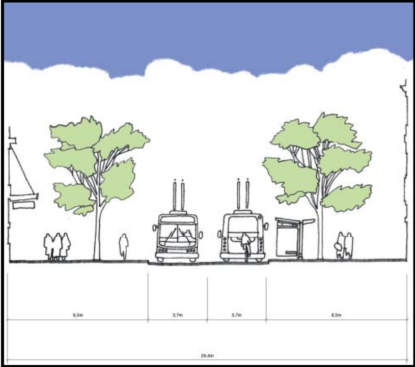
Typical Cross Section north of Smith Street
