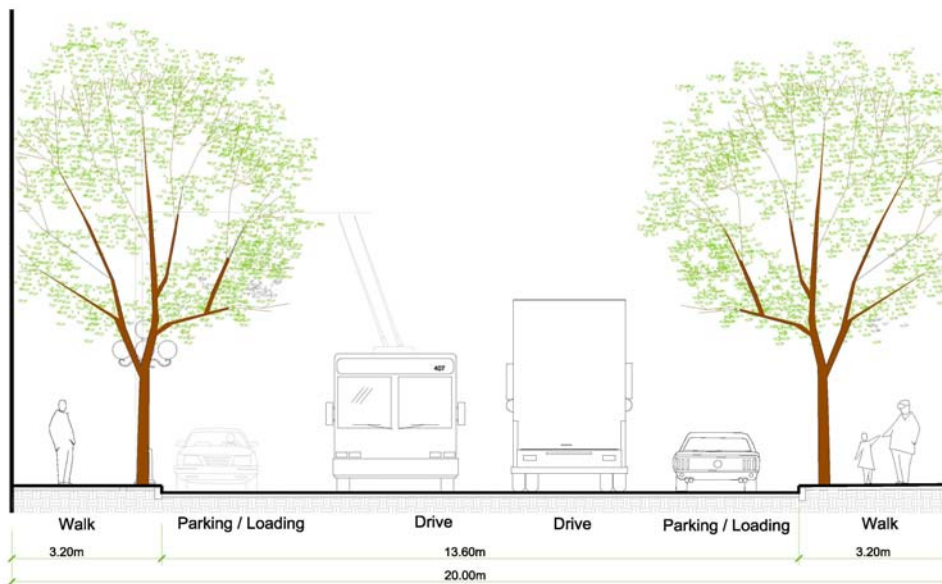
Figure 3: Existing Cross Section (looking north)
