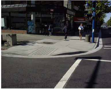
curb ramps - new standard
