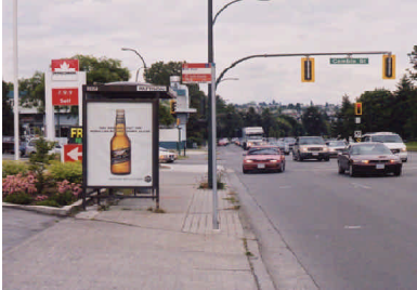
shelter compromises pedestrian corridor
