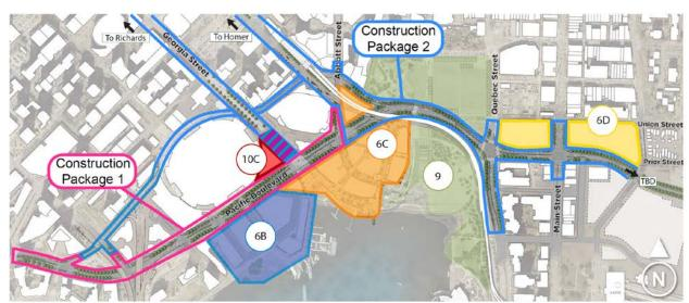
Figure 6: Anticipated construction packaging for integration with development (pink highlights Package 1, blue highlights Package 2, 10C Parkade hatched in pink/blue to be coordinated as Early Works to Package 2)
