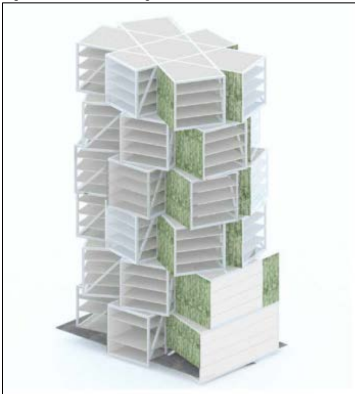
Figure 3 - Cantilevering steel boxes off circular core
