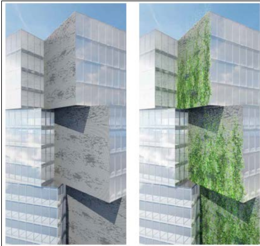
Figure 4 - Living wall growing on expanded mesh
