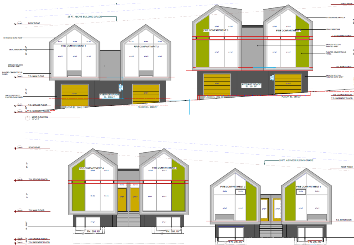
Elevations of New Infill Buildings
