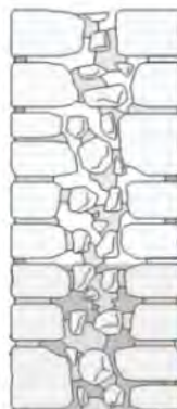
Left and centre: Examples of historic composite walls ( www.buildingconservation.com ); Right: Sandstone blocks at foundation
