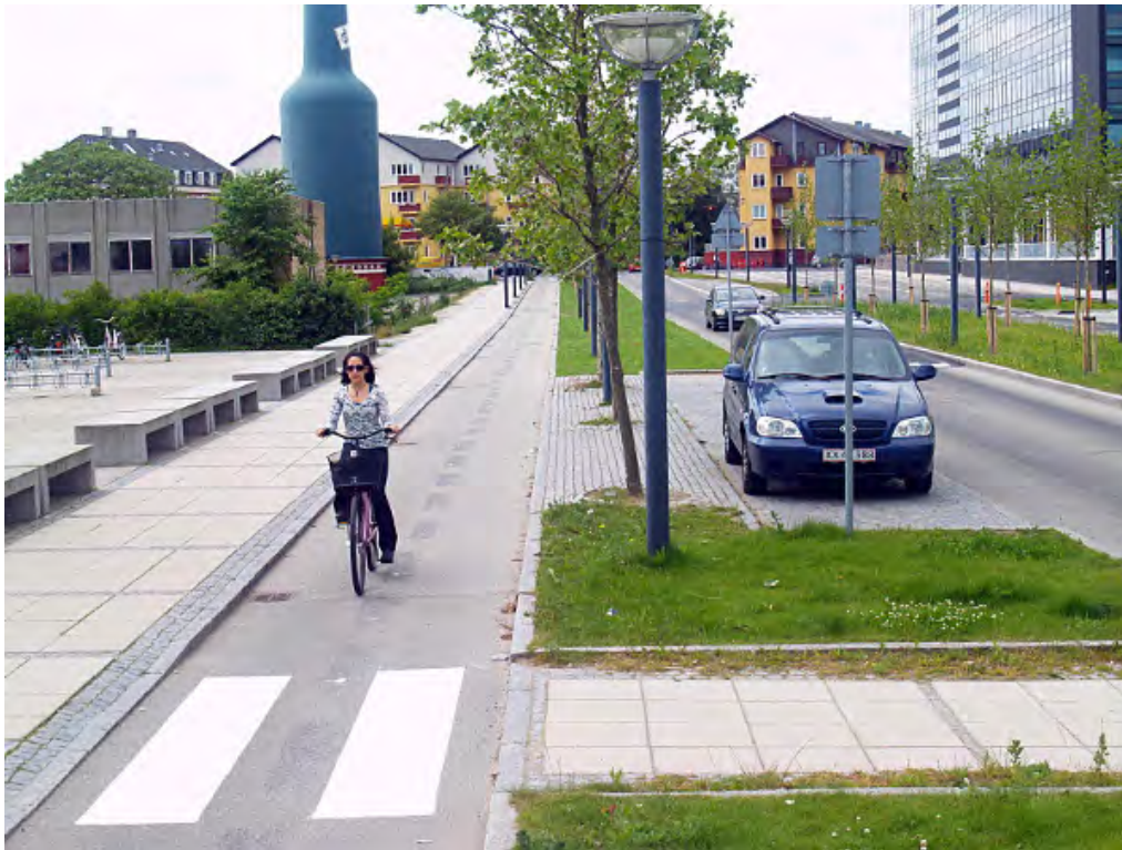
FIGURE 4: ELEMENTS OF A PROTECTED BIKE LANE
