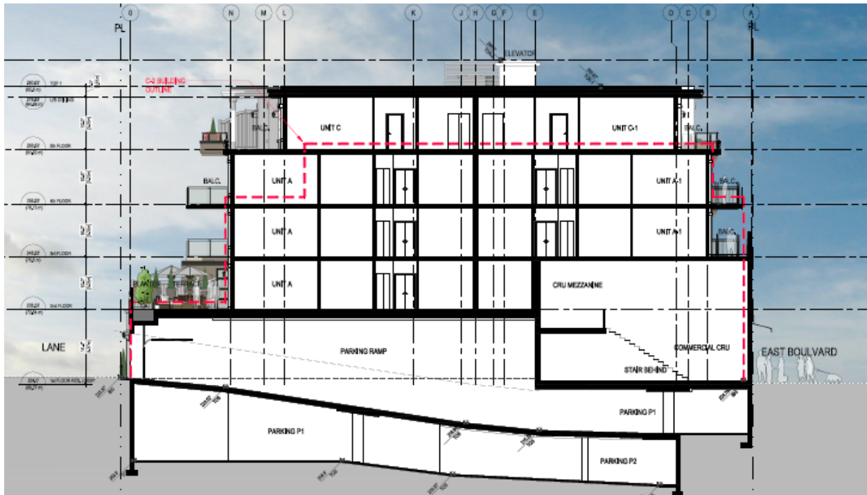
Section Through Parking Ramp (Looking South)
